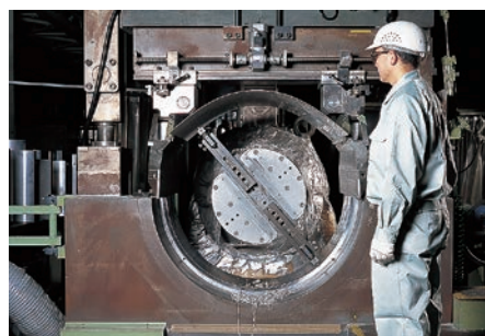
Large-diameter borings Inner diameters of 1000 mm or more are achieved using a high-precision boring process.
